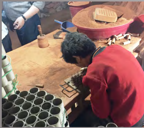
A prep technician places timing fuses and bottom plugs in paper tubes.
